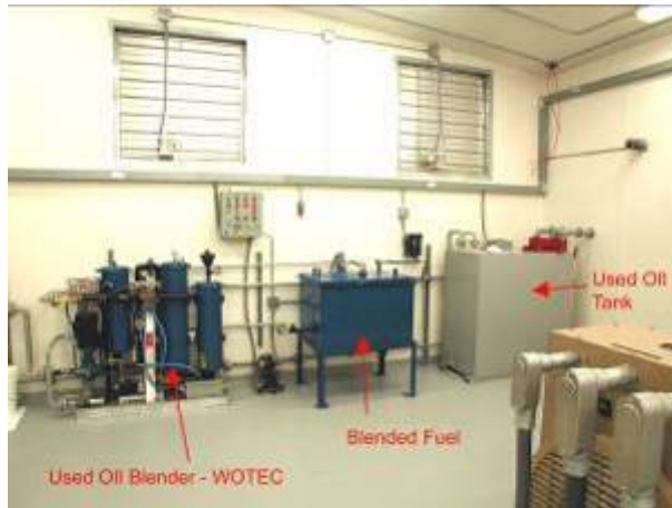
This is a picture of the largest size WOTEC model (15xdc). The initial used oil tank and final blended fuel tank are shown here.
